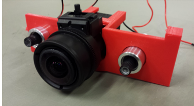
Figure 18: A Point Grey Blackfly GIGE IP camera. Here mounted to a 3D printed frame with lasers attached.
