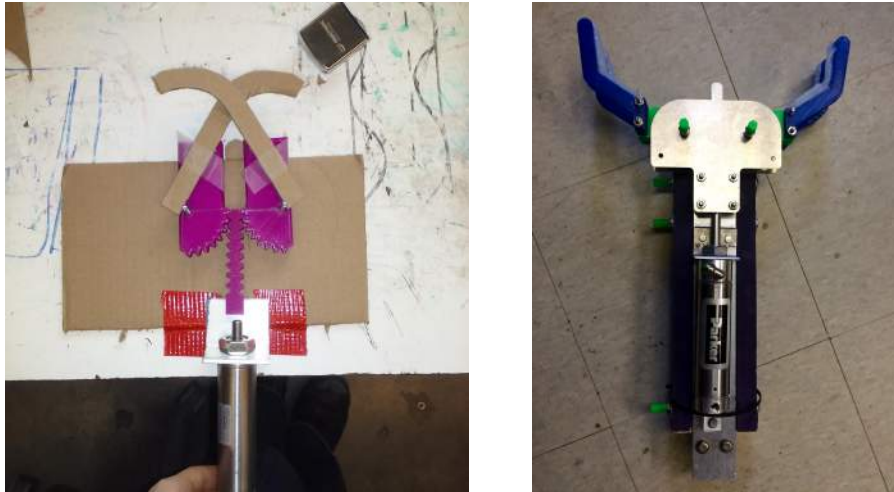
Figure 6. Prototype of manipulator (left) and final product (right).
