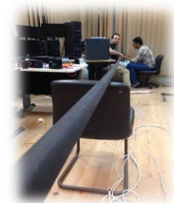
Figure 19: ROV Cables, in heat shrink
