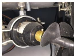
Figure 4: Modified Bilge Pump Thruster
