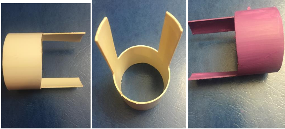
Photo 3: PVC Motor Housing. Photo by Lernisse Collazo
