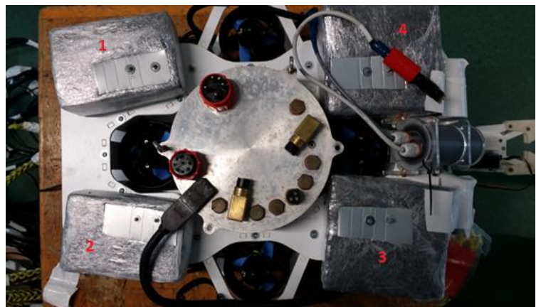
Figure 14 Float placement, indicated by the red numbers
