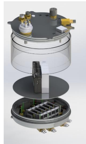
Figure 6 - Exploded view of canister
