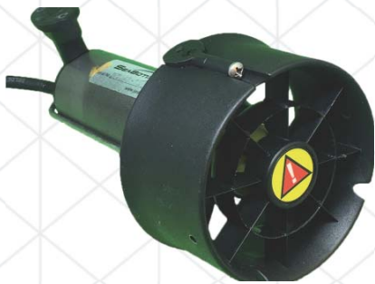
Figure 18: Seabotix thrusters, utilized for forward/backward movement (credit K. Leahy)
