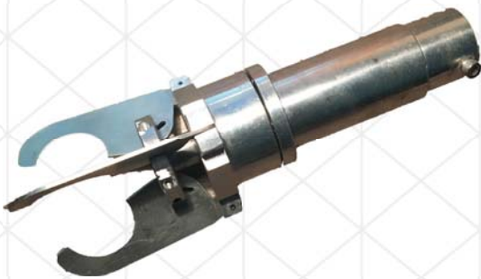
Figure 15: Version 1 of the claw, machined from Aluminum (credit E. Bracht)
