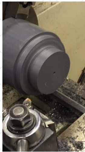
Figure 7-8-: WEH during its machining process.
