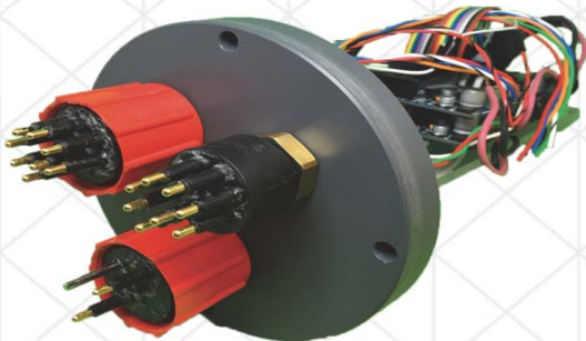
Figure 9: Front/side view of the WEH cap w/ electronics (credit K. Leahy)
