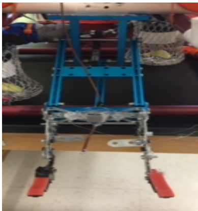
The grey part is the custom designed tusks. The blue is the robotic arm.
