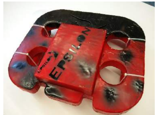
Figure 17: Styrofoam providing 90N of buoyancy
