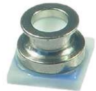
Figure 21: Overview of MS583730BA01-50 pressure sensor
