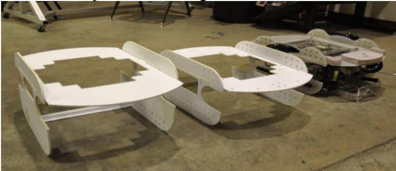
Figure 2: comparison showing laser cut frame mockups next to our final frame.
