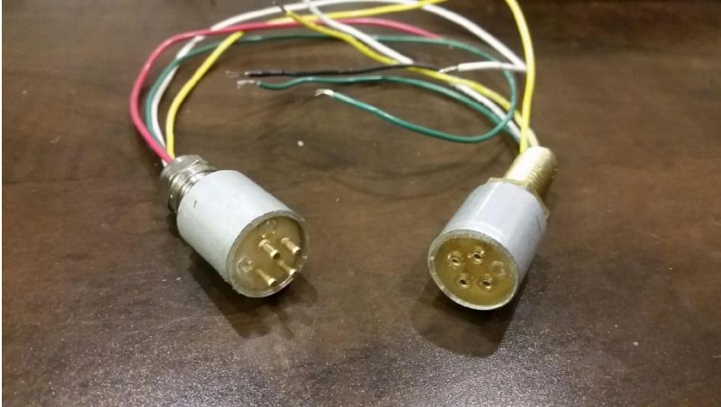
Figure 3: First article test of our waterproof connectors.
