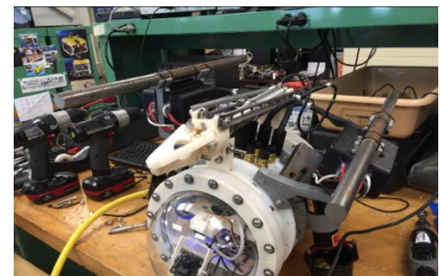
Figure 31: (ROV inverted) custom in-house 3D printed manipulator installed. Also shown are the bulkhead connectors.
