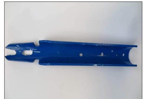
Figure 30: Milled PVC Thomas tool (T-tool) used on the rear side of Seawolf V to assist in mission work.
