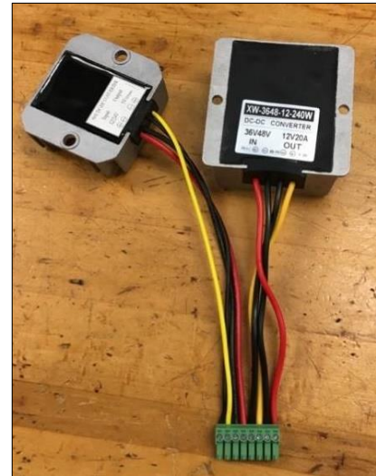
Figure 21: DC - DC step-down converters shown with detachable Wurth connectors
