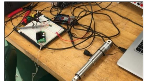
Figure 29: Testing the Concens linear actuator's Hall sensing technology.
