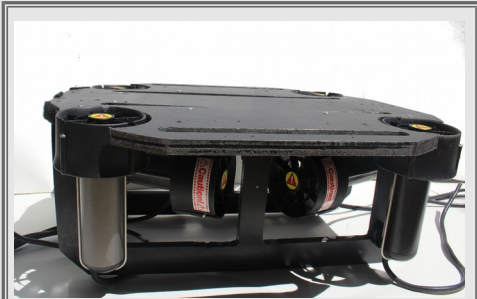
Figure 1: The UHMW frame with the thrusters mounted.
