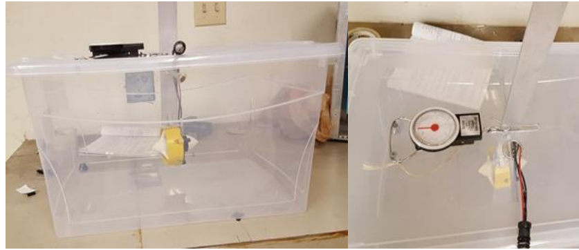
Figure 9- Thrust Test Platform of side and top views
