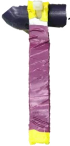
Figure VI: Temperature Sensor with plumbers tape.
