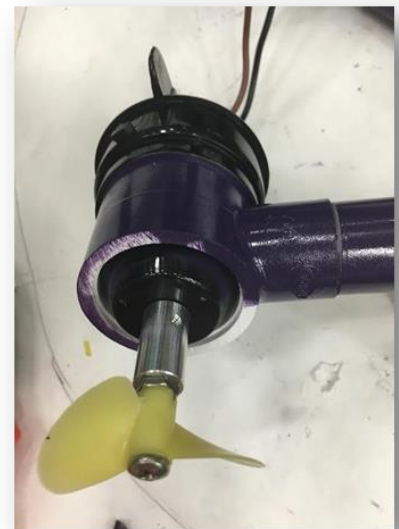
Figure VII: One of Octobot's Johnson 1000GPH motor
