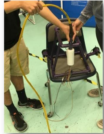
Figure XI: Our tether in the processes of being assembled threw the strain reliever.
