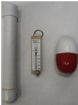
Figure XIV : PVC 3.81cm x 33cm 2 newton's lift Buoy 7.5cm x 12cm 4 newton's lift
