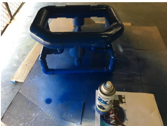
Figure 32: PVC Frame ROV frame being painted.
