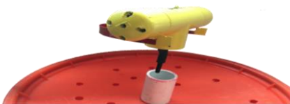
Figure 25: Thermometer The thermometer is designed the same shape and size as an oil sample therefore the Oil Sample Retrieval Tool can work them both effectively.
