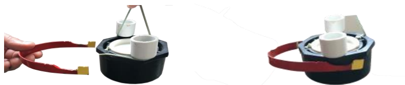
Figure 25 & 26: Retrieving the Well Head Cap The Oil Sample Retrieval Tool is designed to be the exact width of the cap to be lifted from the ocean bottom and installed on the well head.
