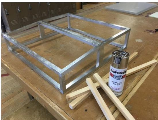
Figure 11: Final Control Box Frame Wood painted metallic color. This creates a strong frame with a modern, finished, appearance within our tight budget.
