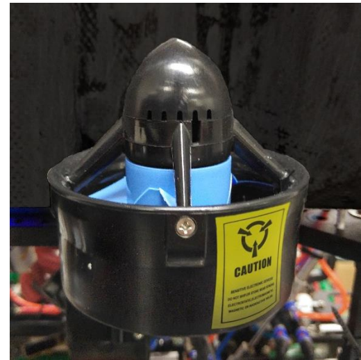
Figure 37 Orca's thruster with safety sticker
