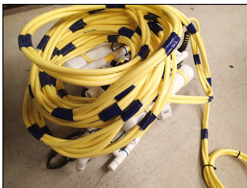
Figure 14: Neutrally buoyant tether (Photo Credit: V. Cariello)
