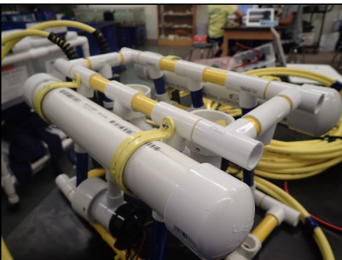
Figure 12: Buoyancy tube placement (Photo Credit: E. Stillman)
