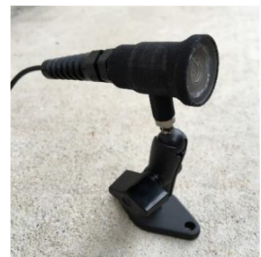
CUSTOM 3D PRINTED CAMERA HOUSING WITH MOVABLE MOUNT
