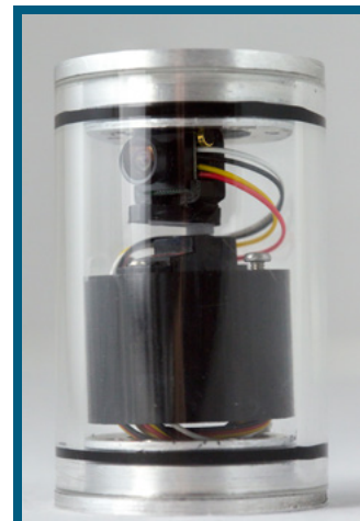
Figure 13. Cuttlefish navigation camera mounted on a servo motor and sealed in its housing.
