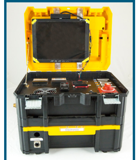
Figure 10. Cuttlefish's TCU and incorporated electronics.
