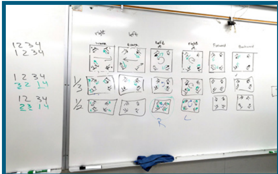
Figure 27. Configuration diagram detailing thruster order and direction.
