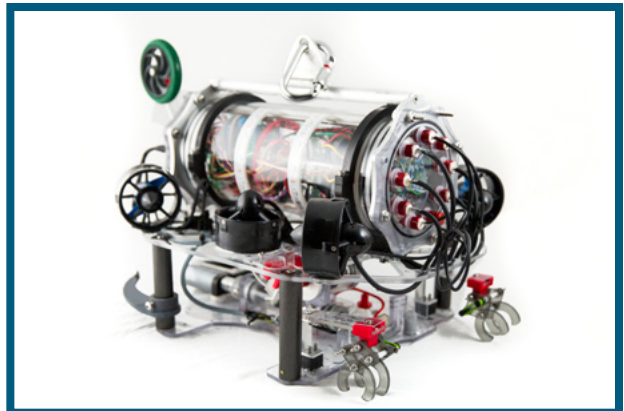
Figure 6. Cuttlefish's frame, fully assembled, with its electronics and thrusters on the top platform and tools on the bottom.
