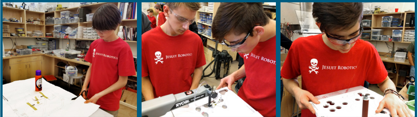
Figure 5. Rovotics' three-step manual frame manufacturing process: preparing a 1:1 paper platform pattern (left); cutting a polycarbonate platform based on the pattern with a bench scroll saw (center); and detail sanding the platform with an oscillating spindle sander (right).
