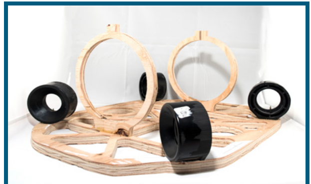
Figure 3. Proof of concept design using PVC parts and wood cutouts.
