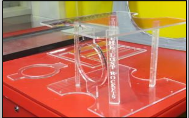
Figure 6: Frame Pieces Before acrylic bonding
