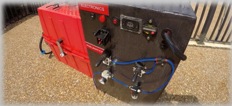
Figure 12: Pneumatic Control System -Mack Van Wagnen
