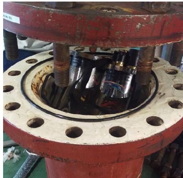
Pressure test chamber used for testing dry housing seals
