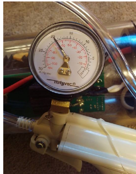
Vacuum pump test setup for doing easy tests of the dry housing's seals
