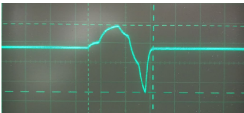
Oscilloscope capture, with 85\text{mF} of capacitance, showing a small 50\text{ms} , 0.5\text{V} spike, with the regulators continuing to function
