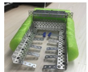
Figure 27: Oil sample capture mechanism
