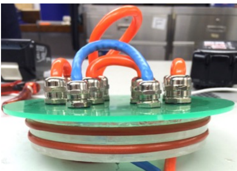
Figure32: The cap of underwater control housing (SolidWork model)
