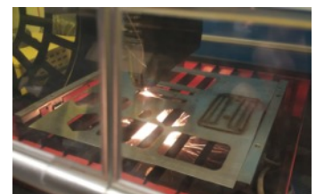
Figure8: Cutting aluminium on metal laser cutter
