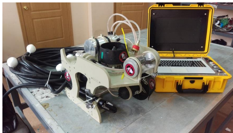
Figure 2 - ROV "Space Wolf" with surface equipment
