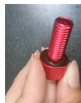
Figure 46: O-rings in the cable penetrators. Captured by Samaa.
