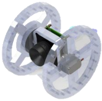
Figure 36: Tilt mechanism of the camera.
