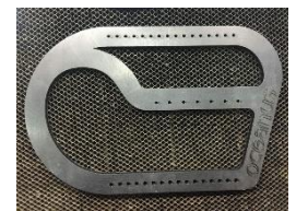
Figure 12: Laser-cut side sheet.
