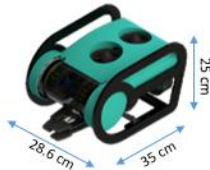
Figure 18: Hera's dimensions. Created by Samaa.
