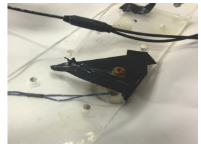
Electromagnet taped to avoid glare in camera
