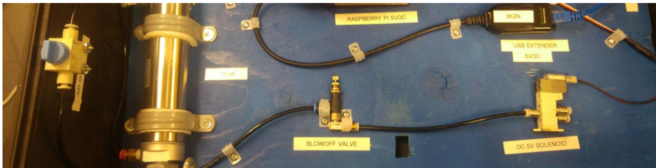
Figure 11: Pneumatic system inside vehicle cockpit using VEX components. (Credit: Sean Purchase)
