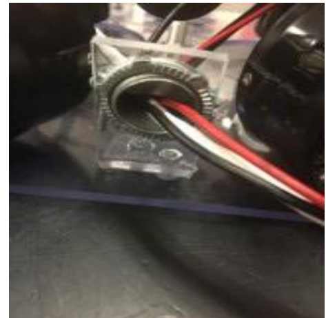
Figure 27: A conduit strain relief is used to secure cables coming from the tether. (Credit: Daniel Drodge)
