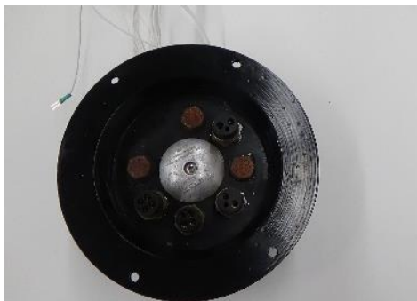
Fig. 11: Sacrificial Anode in End cap Photo: Kraig Kreiner
