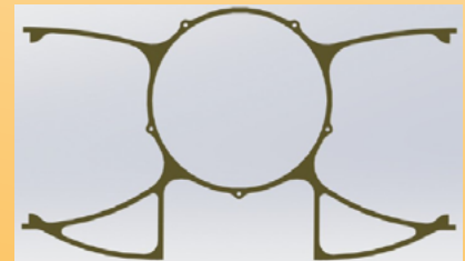
Fig. 6 - One of five horizontal frame plates
