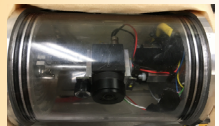
Fig. 10 - Main Camera Housing and Tilt Mechanism
