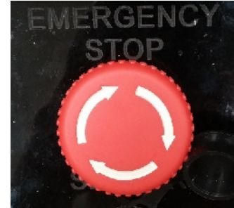
Fig.2b Emergency stop button to terminate the operation of Batfish (Photo Credit: Panda)
