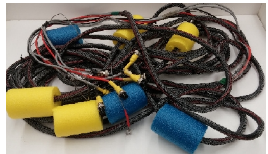
Fig.10 Tether of Batfish is within PET tubing and attached buoys for every meter
