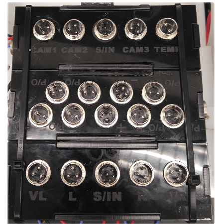
Fig.8a Original Design of on bard Control Box (Photo Credit: Panda)
