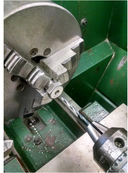
Figure 11: Employee manufacturing a static bulkhead penetrator
