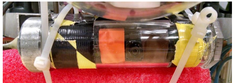
Figure 5: Secondary camera housing configured as a fixed gripper camera.
