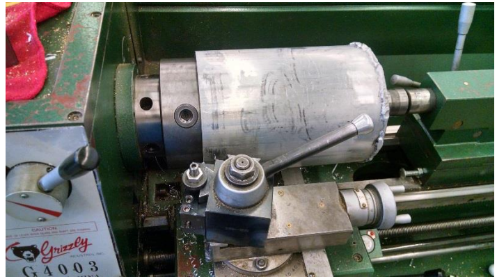
Figure 15: A novel approach to facing the end of the main electronics housing.
