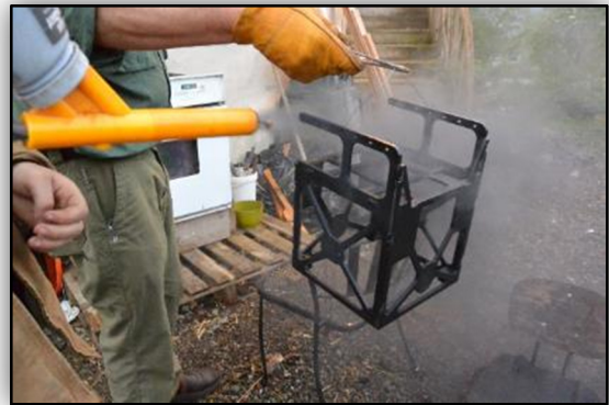
Figure 8 - Powder-coating our Frame
