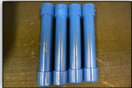
Figure 10 - PVC Filled with Lead Shots for Ballast
