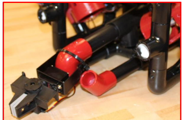
The Admiral's hydraulic powered collection device.
