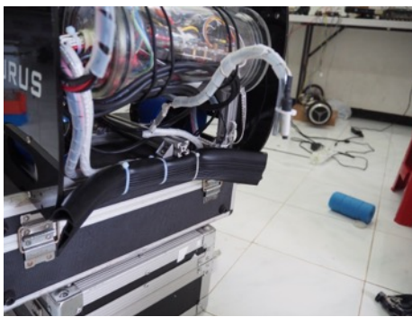
Figure 22: Temperature sensor with rubber guide (Credit: Samuel A.)
