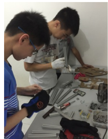
Figure 25: Assembling ISURUS' aluminium frame (Credit: Ghevaldo G.)
