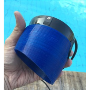
Figure 12: T100 thruster with Jet-drive nozzle (Credit: Samuel A.)
