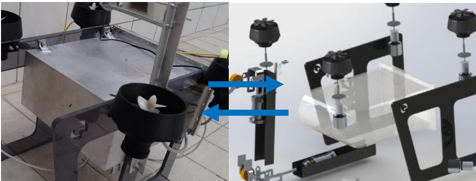
Figure 9 Fuselage – reality (aluminum) and conception (acrylic glass)
