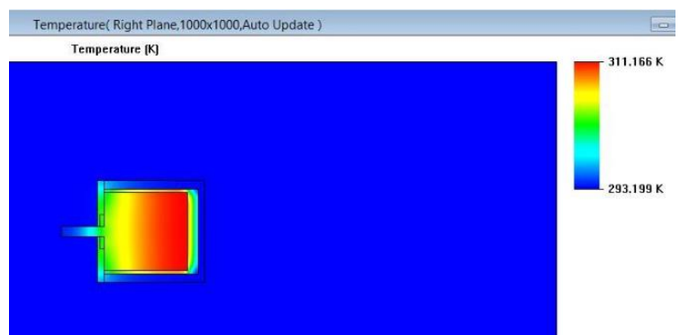
Figure 10 Simulation of the heat distribution within the motor
