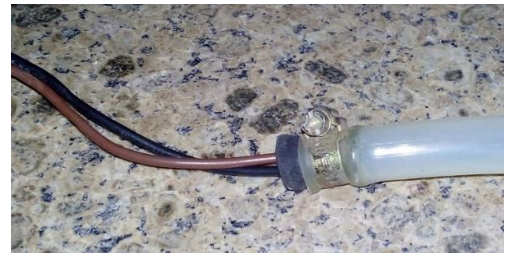
Figure 18. Wire sealing technique.
