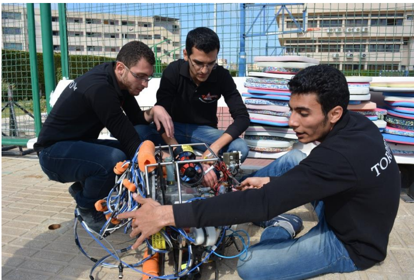
Figure 52. Troubleshooting and adjusting parts of ROV, such as buoyancy.
