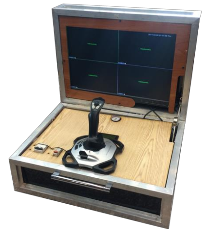
Figure 23. Latro's Tether Control Unit (TCU).
