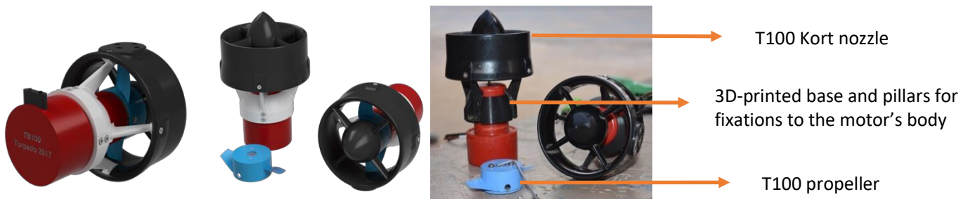
Figure 10. Torpedo's newly developed ROV thrusters(TP100) in CAD (left) and real view (right).
