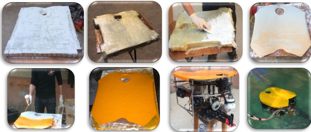
Figure 22. Steps and sequence used to build Latro's fiber glass cover in Torpedo's workshop.
