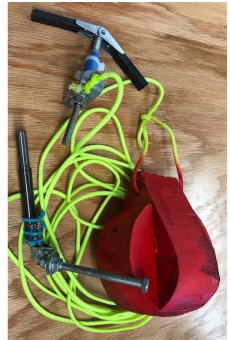
Fig. 16: The bouy and its deployment system.
