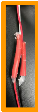
Figure 31 Waterproof solder connection
