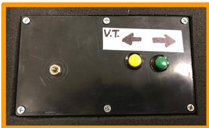
Figure 23 Valve Turner and Claw Control Box
