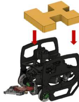
Figure 15: The buoyancy of the buoyancy board neutralizes the weight of Zeta in water with a total of 3.89kg.
