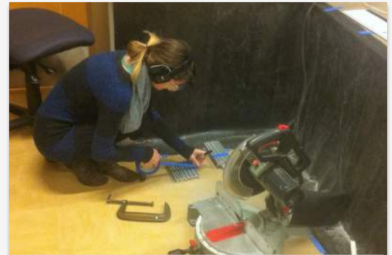
Fig 5.1.1: Trained company members are required to wear PPE when operating the Miter Saw
