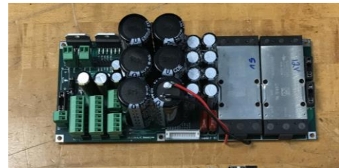
Figure 16 The power supply board consists of multiple Wurth headers for switching circuits which makes adding new equipment an easy task for tooling expansion.
