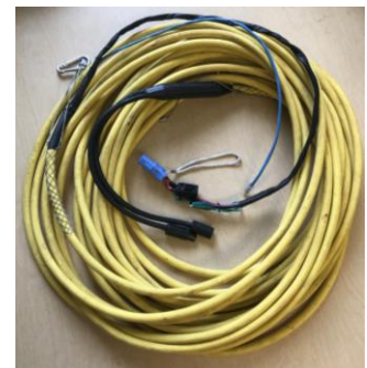
Figure 23 The Outland's Technology tether is already neutrally buoyant and rugged to last in the Port of Long Beach.
