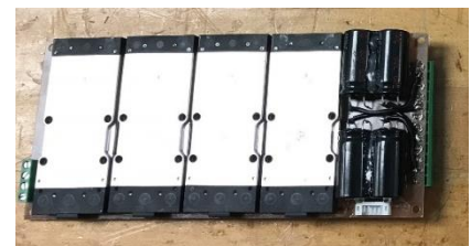
Figure 19 Motor converter board is located on top of the rack and should any trouble arise the outputs are effectively located on the side for any troubleshooting needs.
