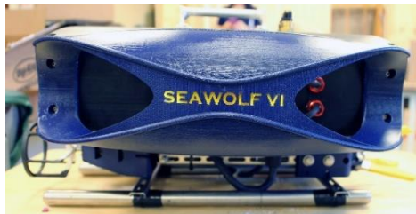
Figure 38 Thruster guards and tooling mounts are 3D printed ABS plastic. The 3D printing process provides a safer and more efficient machine while ensuring personnel safety due to the hands-off nature of production.
