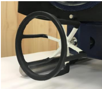
Figure 12 The F.A.R.T. 2.0 was modified from the previous model and utilizes a specially cut PVC cap to turn the valve.
