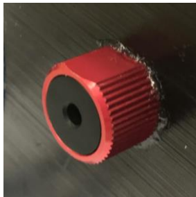
Figure 13 The depth/pressure sensor is located on the front of Seawolf VI.
