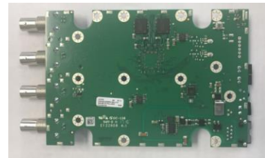
Figure 21 Video Encoder includes four-feed capability, should the need arise the SeaWolf VI has room for expansion with ability to house 2 extras cameras.
