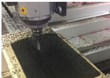
Figure 14 The presence of black shavings intel the milling process of the ROV body from HDPE.
