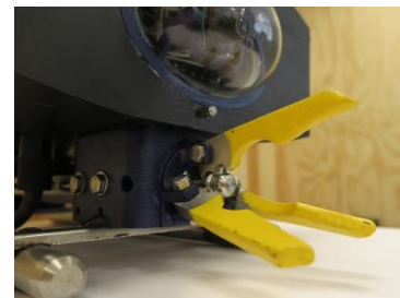
Figure 10 The manipulator is placed under the camera for easy viewing during missions.
