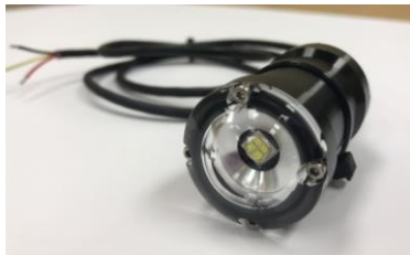
Figure 11 An LED simulates laser needed for soil testing.
