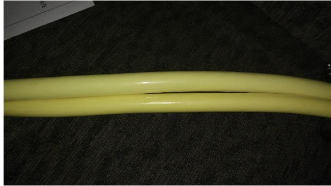
Figure 14- Example of the neutrally buoyant tether
