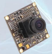
Figure 42: Low-light analog camera used as eagle-eye
