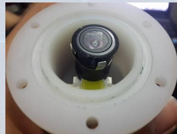
Figure 44: mapping camera inside its water-tight enclosure
