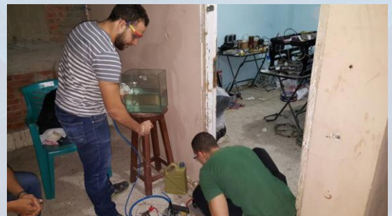
Figure 50: Testing the water-tightness of our enclosures
