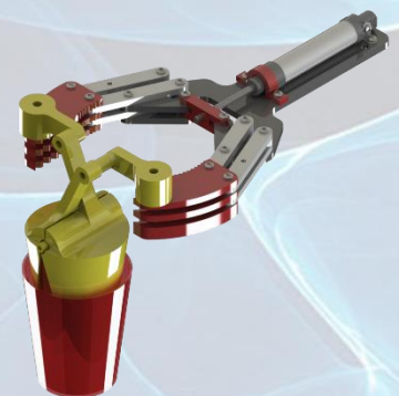
Figure 26: Sediment collecting claw inside a beer cup
