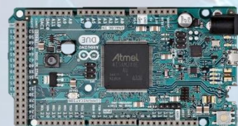
Figure 46: Arduino Due used as V-ray’s microcontroller
