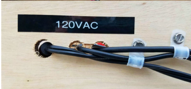
Above and Left: Entrance points for the tether and power. Strain relieved and labeled for safety. (Photo: Roepcke)
