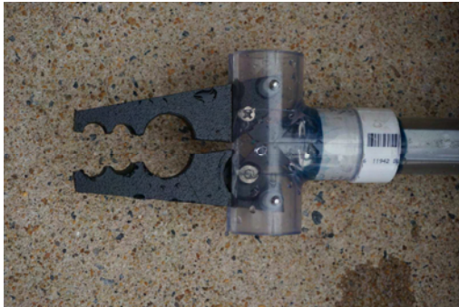
Left: Manipulator. Fingers are driven by an Actuonix DC Linear Actuator. (Photo: Piland)
