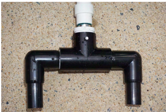
Right: redesigned valve tool. The new tool is shaped to the exact dimensions of the shut-off valve for the fountain. (Photo: Thomas)
