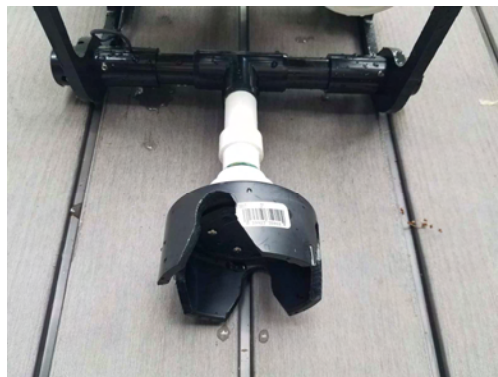
Right: redesigned valve tool. The new tool is shaped to the exact dimensions of the shut-off valve for the fountain. (Photo: Thomas)
