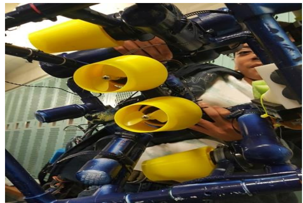
Figure 6: Bilge pump motors featuring 3D printing motor shrouds.
