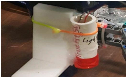
Figure 12: Photo of the raman laser.
