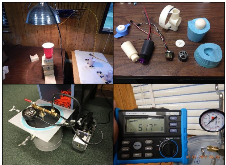
Figure 9: Waterproofing the Motors
