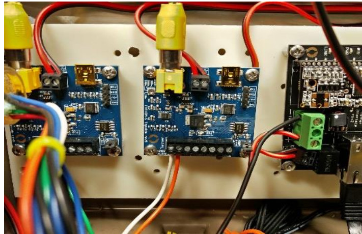
Figure 17: Top-Side Fathom-S and Fathom-X Boards
