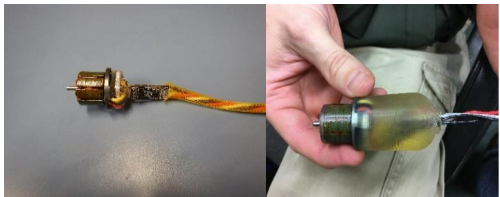
Figure 10: Custom Motor Before and After Potting
