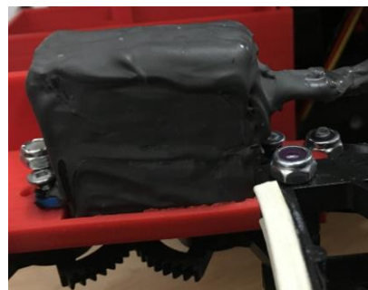
Servo waterproofed to 4m+ and insulated to 100M \Omega +
