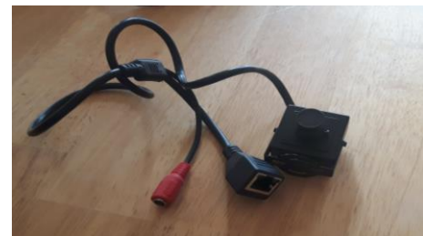
12V IP Camera before re-wiring
