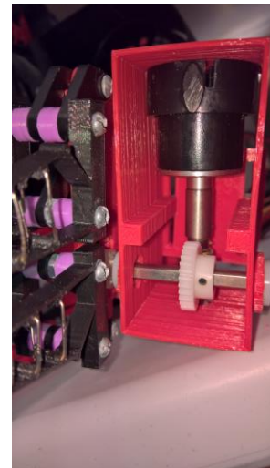
Custom Gearbox with plastic gears/bearings
