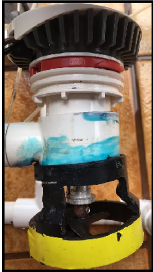
Figure 4: One of Kumu’s four thrusters attached to the frame. (Credit: R. Lee)
