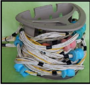
Figure 5: Kumu's tether neatly bundled. (Credit: L. Adcock)
