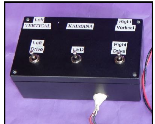
Figure 6: Control box with labels for thrusters and a fuse. (Credit: L. Adcock)
