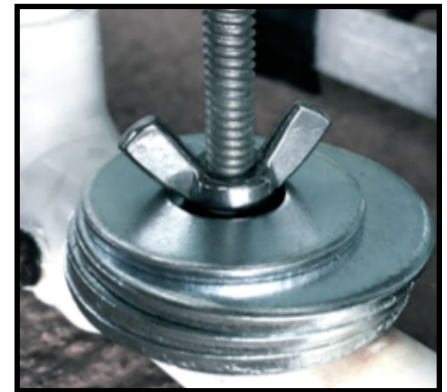
Figure 3: Washers used to easily adjust buoyancy. (Credit: R. Lee)
