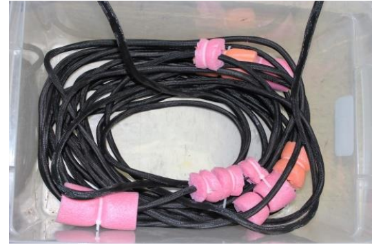
Our tether covered with several pool noodles for buoyancy
