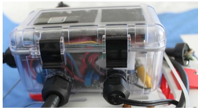
The onboard electronics box with cable glands
