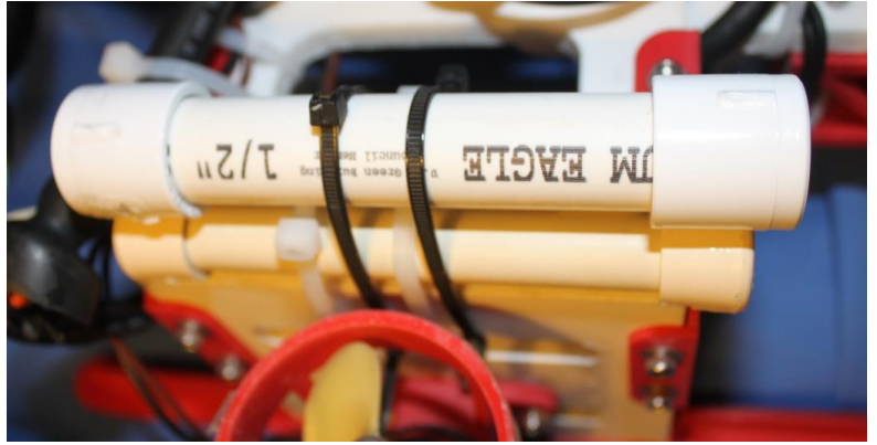
CPVC and PVC pipes attached to the ROV's frame by zip ties
