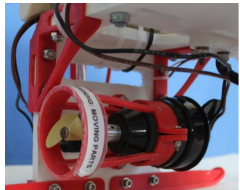
A bilge pump motor attached lower on the frame for ballast
