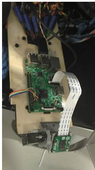
Figure 23 Raspberry Pi Raspberry pi 3 Model B has a 4 core 1,2Ghz processor and 1GB of RAM. Raspberry Pi Camera uses 8Mpx chip
