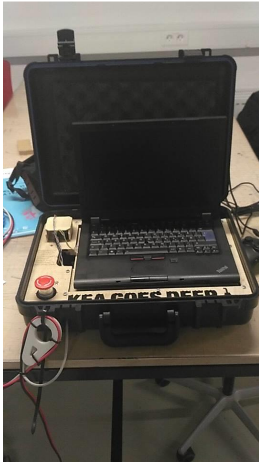
Figure 18 Box with a laptop, ground station and PCB
