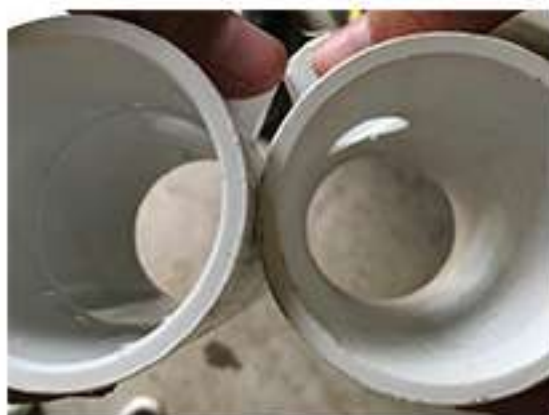
Left: unmodified tee pipe Right: modified tee pipe
