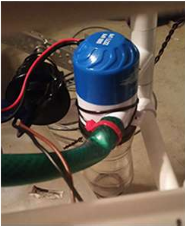
The ROV'S bilge pump.
