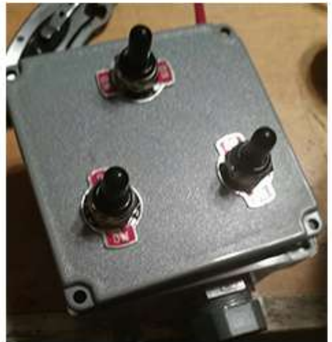
One of the two control boxes used to maneuver the ROV.
