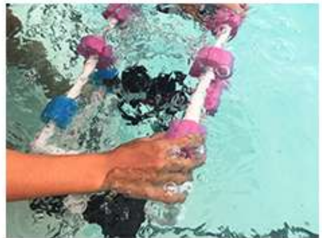
Testing the buoyancy of the ROV in the water.
