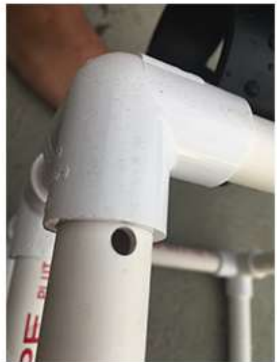
One of the holes in the PVP, used to achieve buoyancy.
