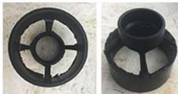
Top and perspective views of one of the modified propeller shrouds
