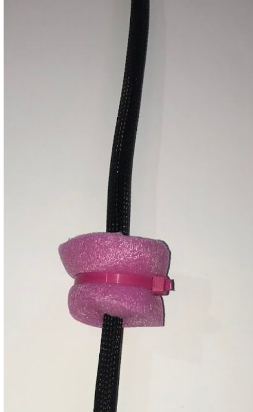
Figure 15. The tethers material and buoyancy device
