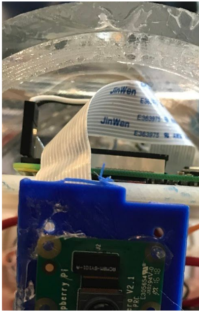
Figure 9. Camera in its housing and attached to the gimbal Figure 10. Back shot of gimbal and servo
